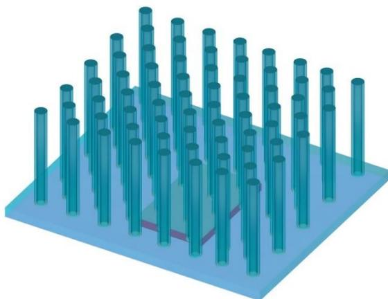
Figure 1: Schematic of a two-phase heat spreader with integrated fins
