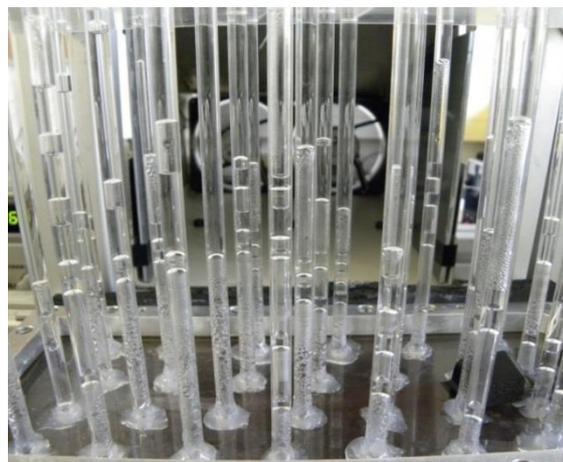
Figure 2: Example of condensation pattern in an array of transparent tube
